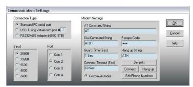
Stingray baud rate is fixed at 28800 and Greyline Logger baud rate must be set at 28800 to match.
