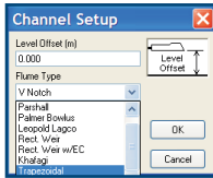
Generates Flow Reports from Flumes and Weirs
